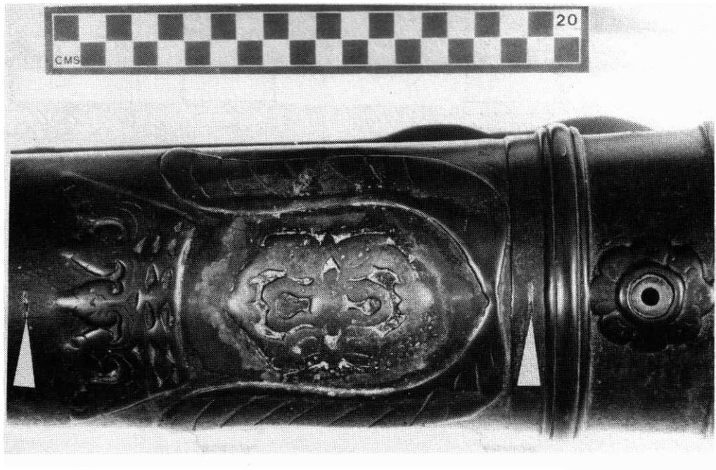
Figure 3. Photograph showing the decorative emblem on the first reinforce and two of the iron chaplets.
